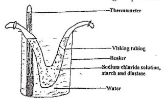
Visking tubing is made of material which acts as a semi-permeable membrane. After some time water from the beaker entered the visking tubing and water in the beaker became salty. The temperature of the experiment was kept between 35°C and 40°C throughout the experiment.
